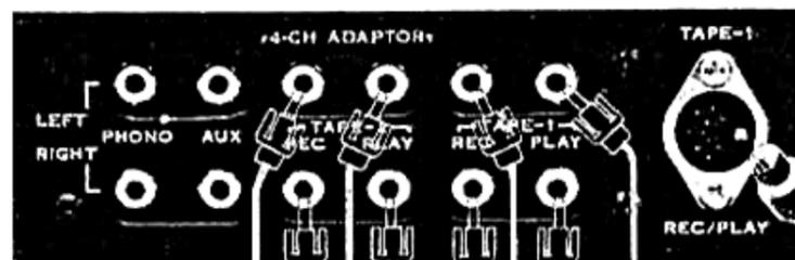
● Do not connect tape deck(s) to TAPE-1 pin jacks and DIN socket simultaneously.
