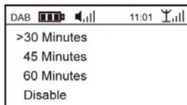
The unit will Power Off automatically after the selected time interval has passed.
