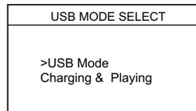
Select <USB Mode> to enter USB mass Storage Mode. You may copy the songs from the PC into the radio and play in MP3 mode. The previous mode will be shown when the USB cable is unplugged.
