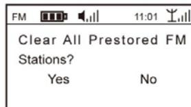
If you confirm and press the **Enter Button**, the radio will clear all the stored stations in the Preset List and Channel List and confirm with 'Clear All', then the radio will go back to the playing screen. To exit without clearing the list, press the **Back Button**
