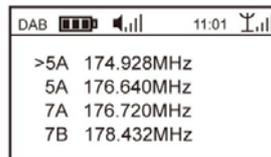
Select a frequency under <Manual Tune>, then press the **Enter Button** to manually search for radio stations on that frequency.
