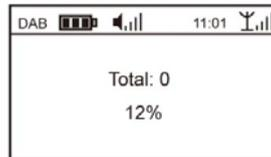
Searches for local stations using the part of band III allocated to the region. When <Local Scan> is selected, the radio will search for radio stations automatically and display the search progress, and when the search is finished, the radio will store the list of DAB stations, and display the number of radio stations found. Then it will play the first station in the list.
