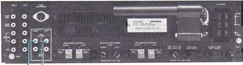
Designed especially for the electronic crossover system, the Sansui 2000A and 3500 stereo receivers are provided with the separate preamplifier section which can be used independently of the power amplifier section. Remove the PM connectors from the 2000A or the 3500, and connect its PRE OUT-PUT's to the inputs of the ECA-3.
