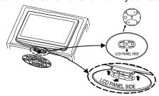
Finally secure the bottom-plate with 2 screws (supplied).
