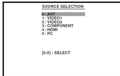
Pressing **INPUT SELECT** on the remote control displays the current signal source. To change the video input source, press **INPUT SELECT** again or 0-5.
