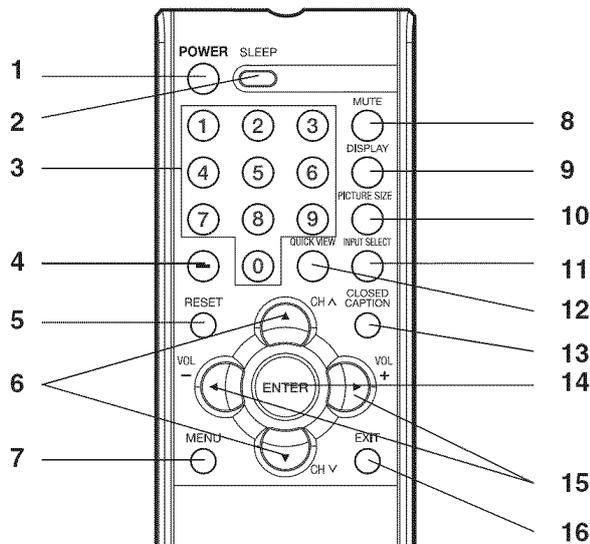
1. **POWER Button** - Used to turn the LCD TV.
