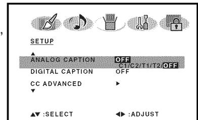
When a Digital signal is received, you can choose from CS1, CS2, CS3, CS4, CS5, CS6 and OFF.
