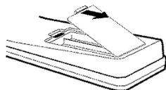
**2** Install two "AAA" batteries, paying attention to the polarity diagram in the battery compartment.
