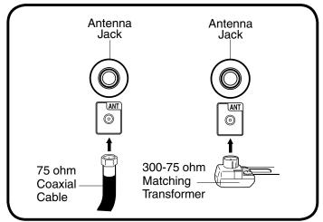
Connect the 75 ohm cable from the combination VHF/UHF antenna to the antenna jack.
