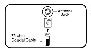
For basic Cable TV service not requiring a Converter/ Descrambler box, connect the 75 ohm Coaxial Cable directly to the Antenna Jack on the back of the TV.
