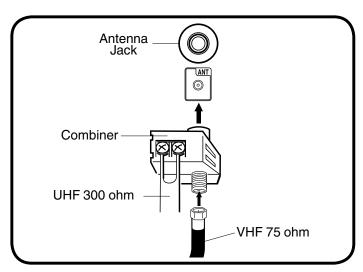
Connect the VHF 75 ohm cable and UHF 300 ohm twin-lead wire to the Combiner (not supplied). Attach the Combiner to the Antenna Jack.
