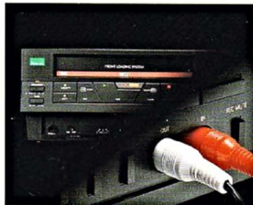
● **Oversized fluorescent meters with peak hold**—Thirteen fluorescent dots per channel show peak levels over a wide 75dB range. Level settings are easy. For one, levels are color coded: white from -60dB to 0dB, yellow
