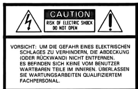
The lightning flash with arrowhead symbol, within an equilateral triangle, is intended to alert the user to the presence of uninsulated "dangerous voltage" within the product's enclosure that may be of sufficient magnitude to constitute a risk of electric shock to persons.
