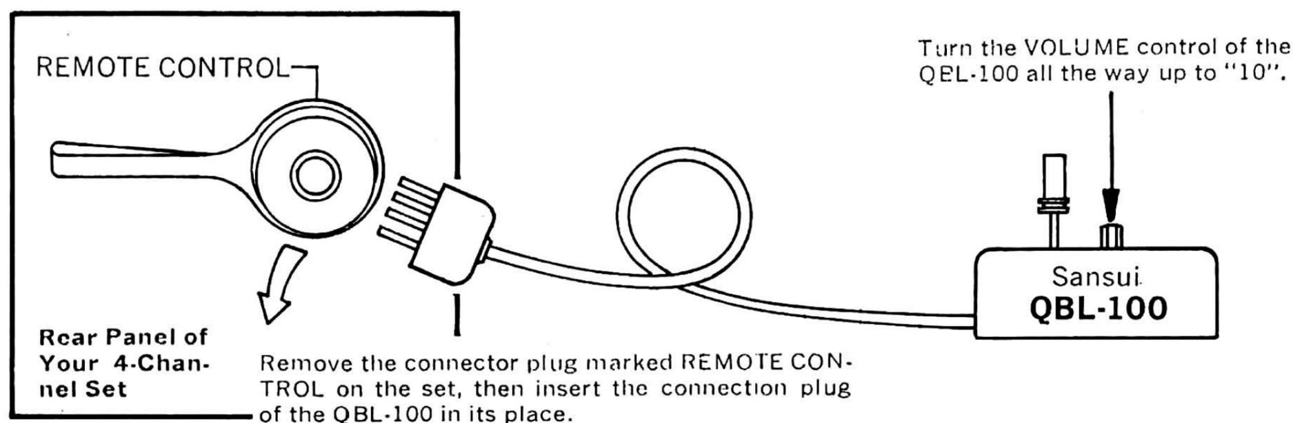
3. Turn on the power switch of the 4-channel set to which you have connect the QBL-100, then its volume control up to appropriate sound volume.
