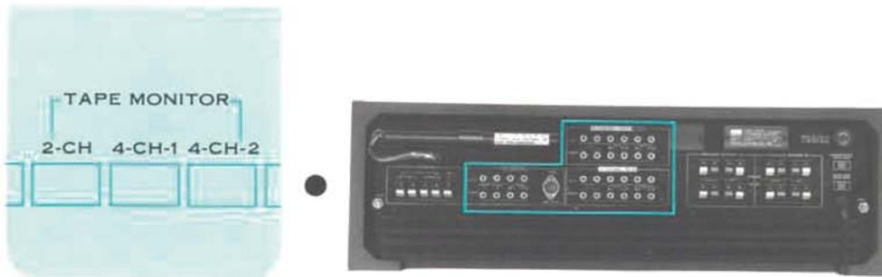
1. Push either the 2-CH, 4-CH-1 or 4-CH-2 TAPE MONITOR switch, depending on which tape playback circuit is connecting the tape deck in use.
