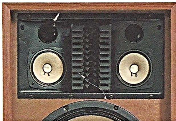
cone speakers has a newly developed concave aluminum dome radiator directly mounted on its voice coil bobbin. This permits a very smooth transition to the tweeters with virtually
