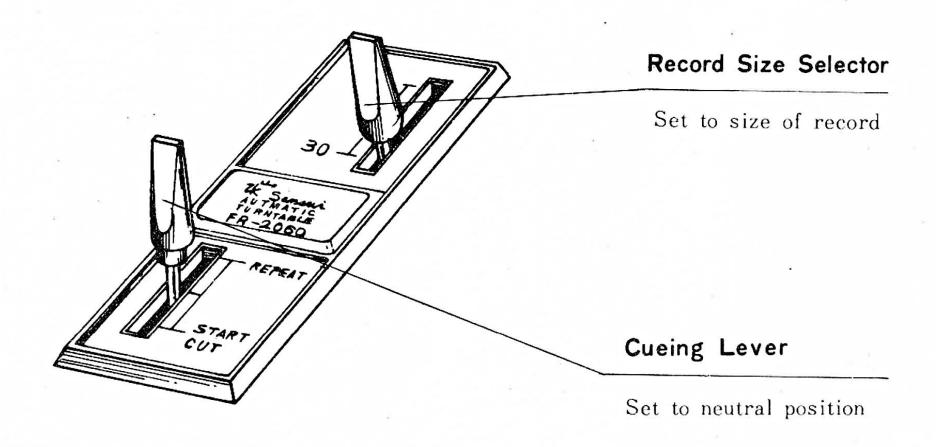
**Caution**: Be sure to set the Cueing Lever to the neutral position without failure. If you leave it in either REPEAT or START/CUT position, the SRC-6 will not work properly.
