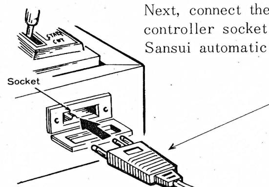
Next, connect the SRC-6 to the remote controller socket on the front of your Sansui automatic turntable, as shown.
