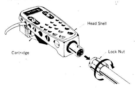
3) Loosen the cartridge retaining screw on the head shell, slide the cartridge back or forth to adjust the overhang. This adjustment is more easily accomplished by following the mounting
