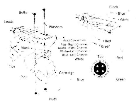
2) Once the cartridge is installed in the head shell, insert the shell into the tip of the tonearm and secure it by turning the lock nut clockwise and tightening it. Pay attention throughout this procedure not to apply unnecessary pressure on the tonearm base.
