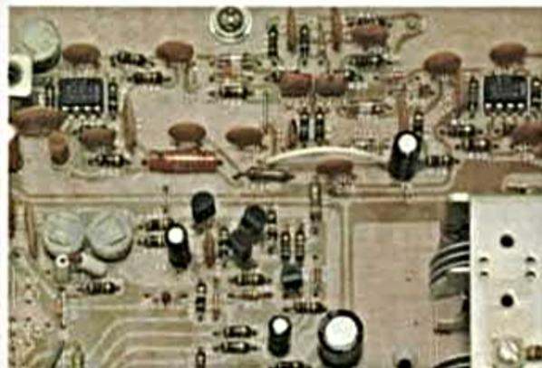
The FM IF input is formed of a low-noise transistor. The following limiting/amplifying stage is where the 10 differential amps, mentioned above, are found. An additional amplifier gives this section 11 different
