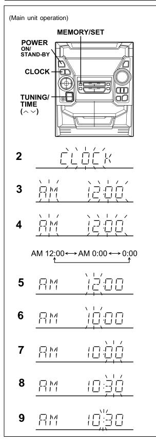
In this example, the clock is set for the 12-hour (AM 12:00) system.
