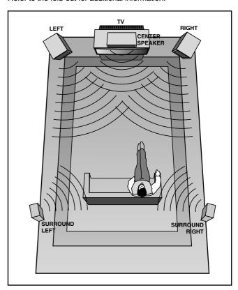
**Note:** to avoid interference with the TV picture, use only magnetically shielded front speaker systems.
