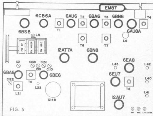
All Sherwood tuners are also adjusted and checked to see that they meet 1/3% IM distortion at 100% FM. To adjust, feed 60 cps; 7kc @ 4:3.35 (equivalent to 4:1 ratio considering standard preemphasis at 7kc.) into a low distortion FM generator. With FM generator rf signal (@ 100% FM) feeding into antenna terminals, read IM distortion at audio output with tuner tuned for zero AFC volts. Adjust T4 (top) for minimum distortion.
