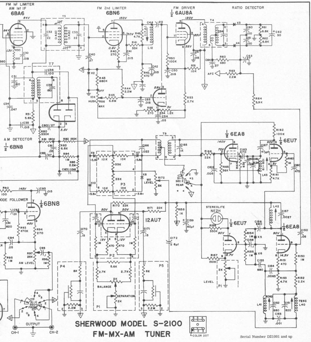
NOTES: All resistors are 1/2 watt,  $\pm 10\%$  tolerance unless otherwise specified. All fractional-valued capacitors are in  $\mu\text{f}$  and are 400v molded paper; other capacitors, except electrolytics, are in  $\mu\text{f}$  and are mica or ceramic.
