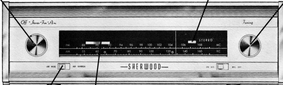
AM selectivity switch. Normally set to left, will reduce static, noise, or interference (as well as fidelity or treble tones) if switched to right.
