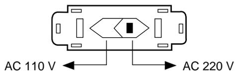
Move switch lever to match your line voltage with a small screwdriver or other pointed tool.
