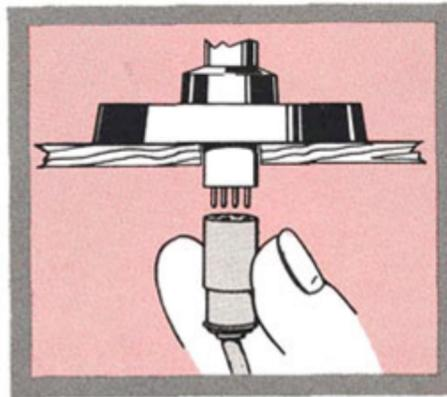
Cable-Plug Assembly Eliminates Soldering
