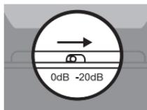
The pad switch helps prevent distortion from extremely loud sources, such as when close-miking horns or drums.
