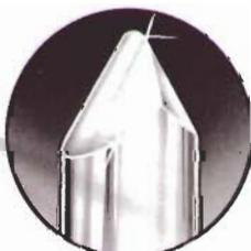
**The Hyperelliptical (HE) Design** is an improvement over all other tip shapes. It is today's state-of-the-art design. The area of the tip that actually touches the record groove wall is longer and narrower than any other shape. This allows it to reproduce sounds with less distortion.
