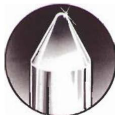
**The Elliptical Design** is considered an improvement over the spherical shape. The elliptical tip is elongated, like an oval. It fits the record groove undulations better than the spherical tip. This means more faithful tracing especially at higher frequency ranges, with less distortion. And the elliptical design can work well with the newer, more lightweight tonearms and cartridges.
