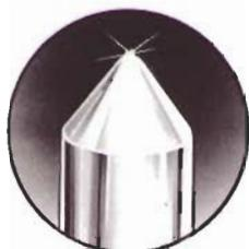
**The Spherical Design** was the earliest design and is probably the most common in use today. A spherical stylus has a simple, rounded tip. It is also called a conical tip. It was particularly well-suited to the early LP recordings, and pre-stereo records, although it is compatible with stereo recordings too.
