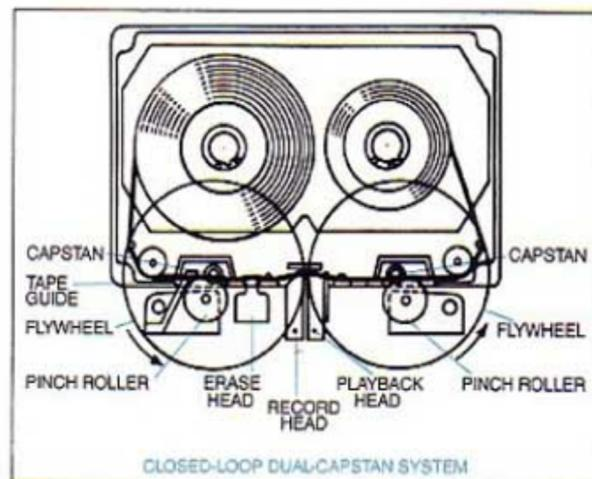
single-capstan drive often yields good performance, dual-capstan drive—using two capstans and two pinch rollers—is a superior system. The TC-K71 and K81 incorporate dual-capstan drive. Both capstans are driven from the BSL motor by the same belt, in a closed-loop configuration. The capstans are located on either side of the head assembly, for better control of tape tension, and minimum modulation noise.
