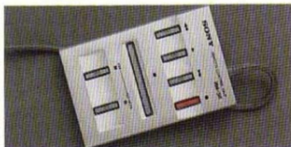
touch pushbuttons provide convenient, foolproof mode selection. You can go quickly from one mode to another, without going through Stop. The logic circuit checks each command for proper sequencing, and protects the tape and mechanism from undue stress.
