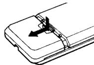
**2** Insert two size AA(R6) batteries with correct polarity.
