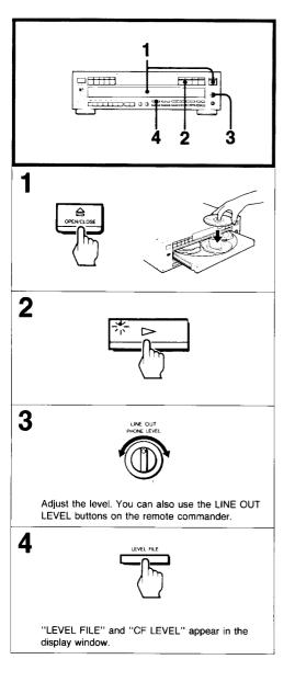
Using the level file function, you can preset the desired output level for each disc. When a disc with the level file is played, the LINE OUT/PHONE LEVELcontrol on the front panel is automatically adjusted to the preset level. When you use the level file function, use headphones or the amplifier connected to the variable line output jacks. This function does not work for the output level of the fixed line output and optical digital output jacks.
