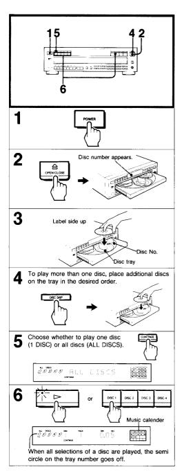
Before playing a disc, turn on the amplifier and set the input selector to the CD player position.
