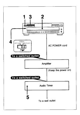
By connecting a commercially available timer, disc play can be started at any desired time.
