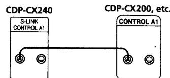
For details on this connection, refer to the supplementary "S-Link™ / CONTROL-A1 Control System" instructions.
