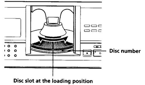
The disc number at the loading position appears in the display.\* If the disc has the Disc Memo (see page 23), the Disc Memo appears instead of the disc number. As you turn the JOG dial, the disc number or the Disc Memo changes.
