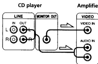
When connecting to an amplifier without a video input jack
