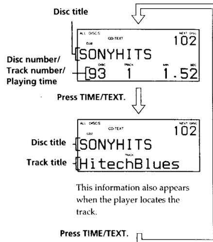
If you have not labeled the track (see "Labeling each track" on page 24), the front panel display information does not change when you press the TIME/TEXT button.
