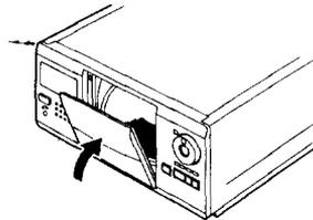
The rotary table turns and the disc slot at the loading position is set to the playing position. Always keep the front cover closed except when you insert or remove discs.
