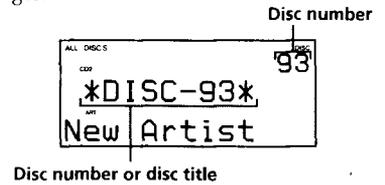
\* If you have already inserted discs, the disc number at the playing position appears. When you turn the JOG dial, the displayed disc number changes to the one at the loading position.
