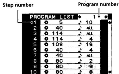
The program number (1, 2 or 3) you are checking appears in the upper right corner of the on-screen display.
