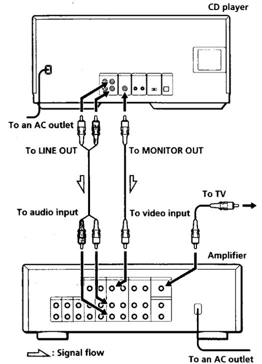
When connecting to an amplifier without a video input jack
