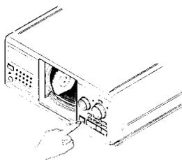
The rotary table turns and the disc slot at the loading position is set to the playing position. Always keep the front cover closed except when inserting or removing discs.
