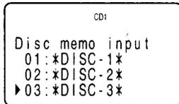
3 Move the cursor to the disc you want to assign a Disc Memo, then press the Easy scroll key. The flashing cursor (◀) appears.
