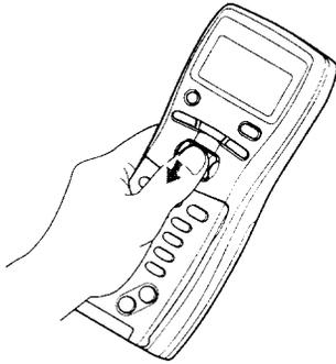
To move the cursor up, push the Easy scroll key upward as illustrated below.
