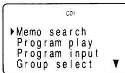
**2** Move the cursor ( $\blacktriangleright$ ) to "Group select" by using the Easy scroll key, then press the Easy scroll key.
