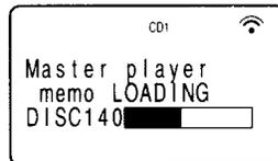
When you want to load each Disc Memo data independently, move the cursor to the data you want to load, then press the Easy scroll key.
