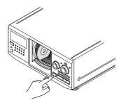
The rotary table turns and the disc slot at the loading position is set to the playing position. Always close the front cover except when you insert or remove discs.
