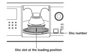
The disc number at the loading position appears in the display. If the disc has the Disc Memo (see page 24), the Disc Memo appears instead of the disc number. As you turn the JOG dial, the disc number or the Disc Memo changes.
