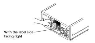
After inserting the disc, you can input the original disc titles instead of the disc numbers (see "Labeling Discs" on page 24) to locate it easily when you start playing.
