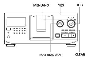
**1** Turn the JOG dial until the disc number to which you want to assign a Disc Memo appears in the display.
