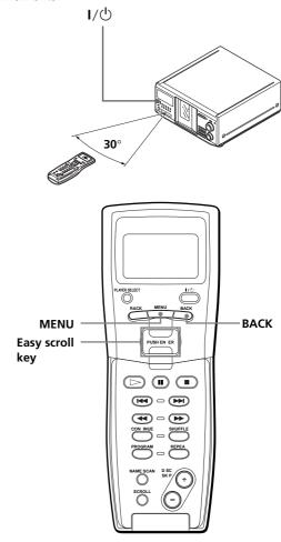
You can select an item shown in the remote's display by moving the cursor (▶). To move the cursor down, push the Easy scroll key downward. To move the cursor up, push the Easy scroll key upward.
