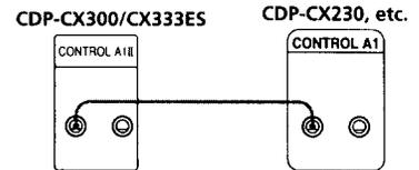
For details on this connection, refer to the supplementary "CONTROL A1 II Control System" instructions.
