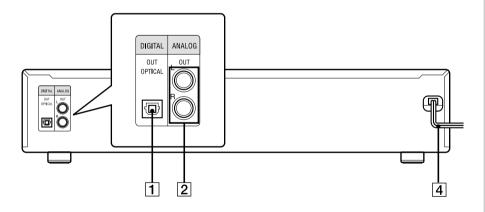
ANALOG OUT L/R jacks 2 (7) CONTROL AIII jacks 3 (8, 15) DIGITAL OUT OPTICAL jack 1 (8) Mains lead 4 (7)
