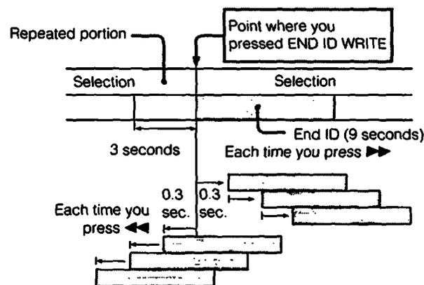
Normally, the repeated portion is played back 5 times. When the **◀◀** or **▶▶** button is pressed while the repeated portion is played back, the repeated portion is played back up to 8 times max, and then tape stops.
