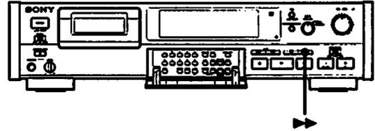
If the previous recording was applied to the middle of the tape, you must locate exactly the last point of the recorded area, and start the new recording from this point. This will prevent leaving a blank section on the tape. If you want space between the last recording and the new recording, use the **REC MUTE** button to mute the sound.
