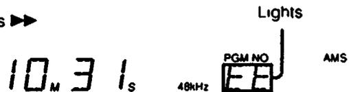
The last point of the previous recording (the beginning of the blank section or the beginning of the end ID\*) is located, and the tape stops. When the end ID is detected, the "EE" indicator lights at the PGM NO. display.
