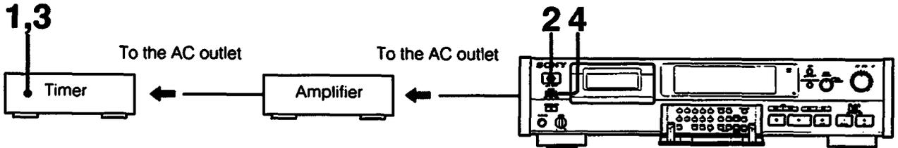
Use a commercially available audio timer to activate recording or playback at a desired time. Read the operating instructions for the timer and the amplifier.
