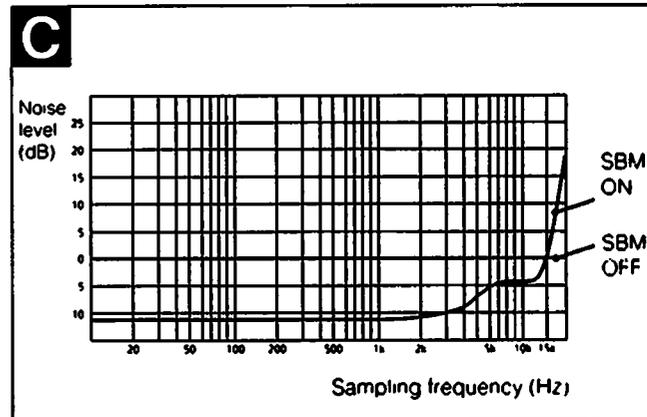
The SBM function operates only during recording. The improved sound produced by the SBM function, however, can be enjoyed during playback, regardless of the SBM switch position or the DAT deck being used.
