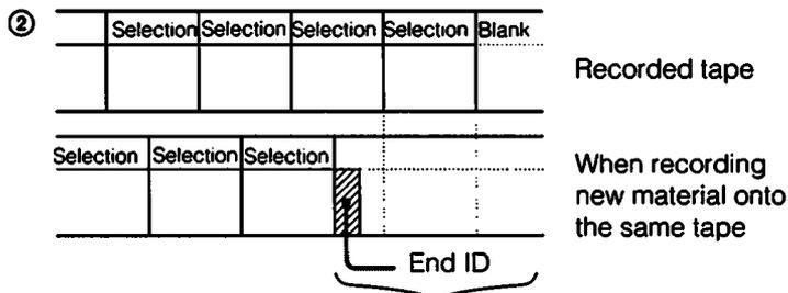
Portion where you have not made a second recording (This first recording has not be erased.)
