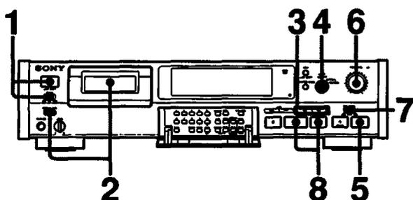
**1** Make sure that the **TIMER** switch is set to the **OFF** position, and turn on the power.
