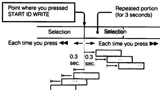
Normally, the repeated portion is played back 5 times. When the ◀◀ or ▶▶ button is pressed while the repeated portion is played back, the repeated portion is played back up to 8 times max, and then tape stops.
