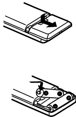
Insert two size AA (R6) batteries with correct polarity, and close the lid.
