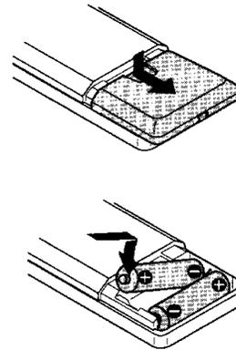
Insert two R6 (size AA) batteries with correct polarity, and close the lid.
