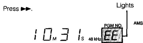
The last point of the previous recording (the beginning of the blank section or the beginning of the end ID\*) is located, and the tape stops. When the end ID is detected, the "EE" indicator lights at the PGM. NO display.
