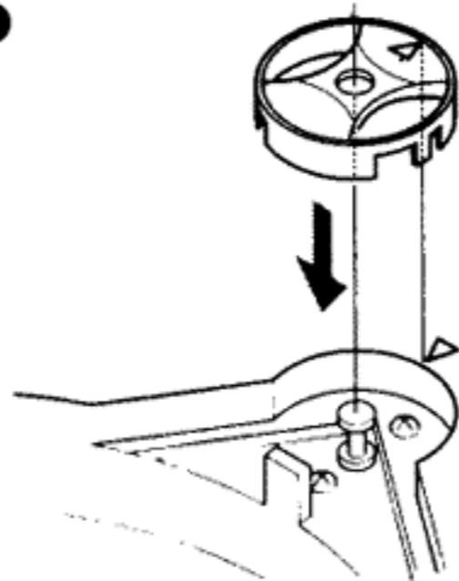
1 Turn the large plastic gear counterclockwise until the notch aligns with the small plastic gear.
