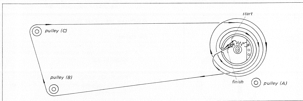
Fig. 2-19 Dial pointer driver cord stringing
