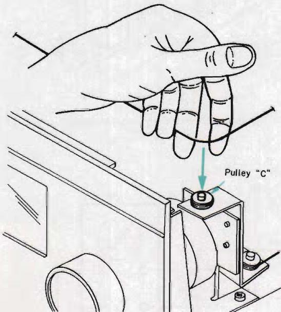
Fig. 2-13 Threading the dial cord over pulley "C"
