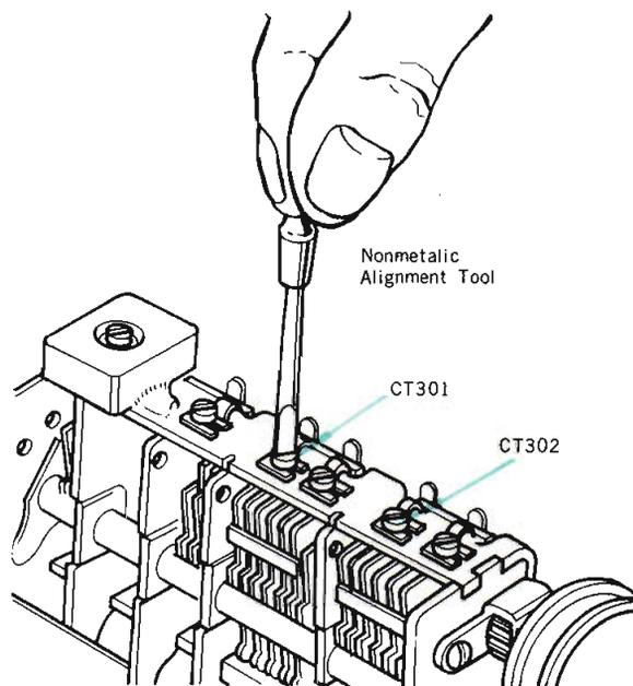
Fig. 3-15 Location of trimmer capacitor CT301 & CT302
