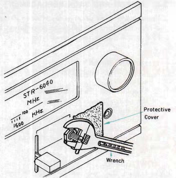
Fig. 2-3 Removal of hexagonal nut
