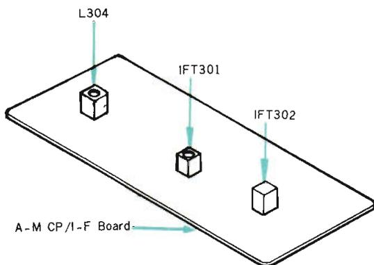
Fig. 3-14 Location of a-m oscillator coil L304
