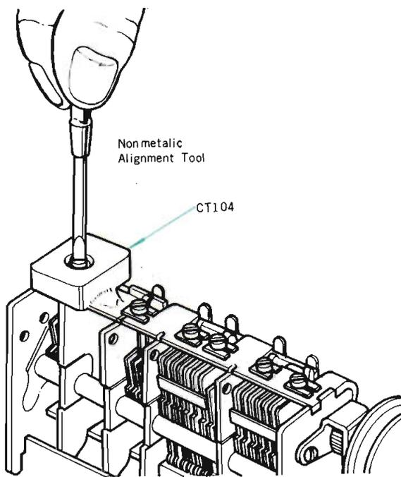
Fig. 3-8 Location of fm trimmer capacitor CT104
