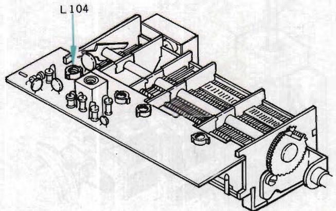
Fig. 3-7 Location of fm oscillator coil L104
