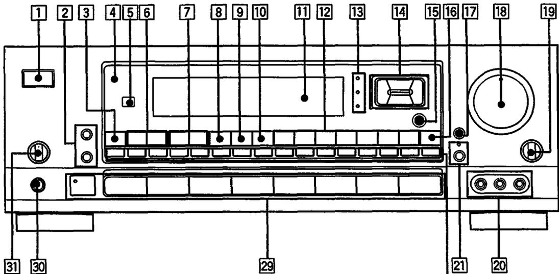
This illustration shows the STR-D911. The STR-D711 is not equipped with the EDIT VIDEO and VIDEO 3 buttons and VIDEO 3 INPUT jacks.
