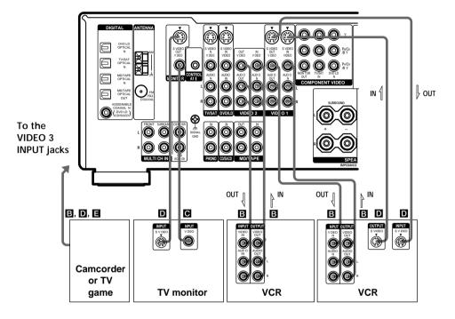
**Tip**When the component is equipped with S-video jacks, you can connect the component to the S-VIDEO jacks on this receiver.
