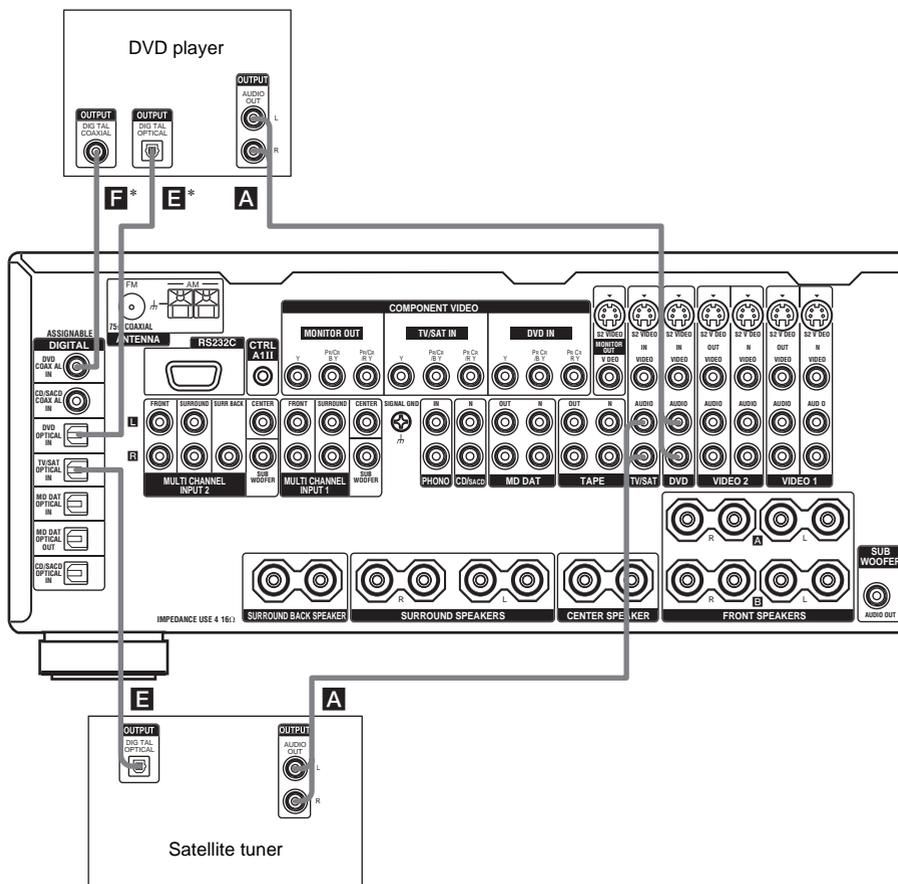
\* Connect to either the DVD COAXIAL IN or the DVD OPTICAL IN jack. We recommend making connections to the DVD COAXIAL IN jack.
