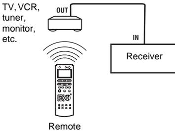
The remote sensor on the CTRL S OUT component receives remote codes the same way as the remote sensor on this unit. This is useful if you have placed this unit in a rack, etc.
