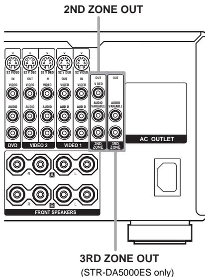
You can select analog audio/video signals for output to the 2nd zone or audio signals for the 3rd zone (STR-DA5000ES only). For details on the connection, see page 53.
