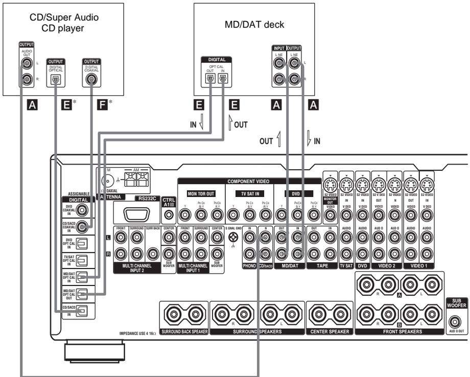
\* Connect to either the CD/SACD COAXIAL IN or the CD/SACD OPTICAL IN jack. We recommend making connections to the CD/SACD COAXIAL IN jack.
