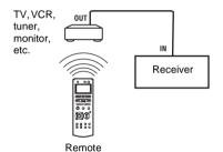
The remote sensor on the CTRL S OUT component receives remote codes the same way as the remote sensor on this unit. This is useful if you have placed this unit in a rack, etc.
