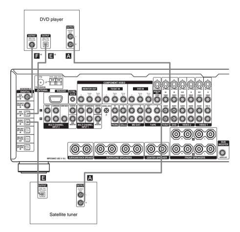
\* Connect to either the DVD COAXIAL IN or the DVD OPTICAL IN jack. We recommend making connections to the DVD COAXIAL IN jack.
