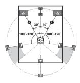
When placing two surround back speakers (The angle <sup>(3)</sup> should be the same)
