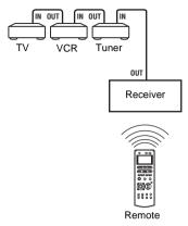
The remote sensor on this unit receives remote codes the same way as the remote sensor on the CTRL S IN component. This is useful if you place the other component away from this unit.
