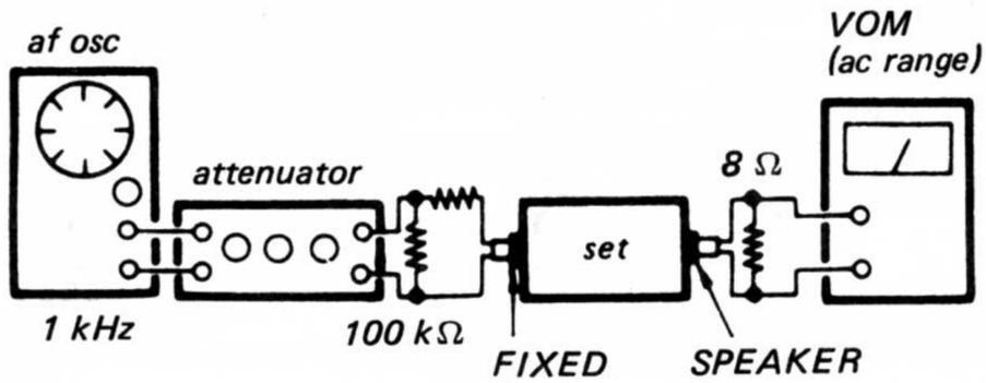
1. Set FIXED input level for 8.9 V reading on the VOM.
