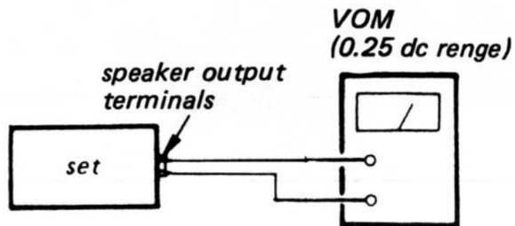
Adjust RT401 (L-CH) and RT-451 (R-CH) for 0 V reading on the VOM.
