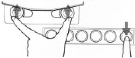
● Don't push the pinch rollers excessively. Too much pressure will deteriorate or even cut the tape.
