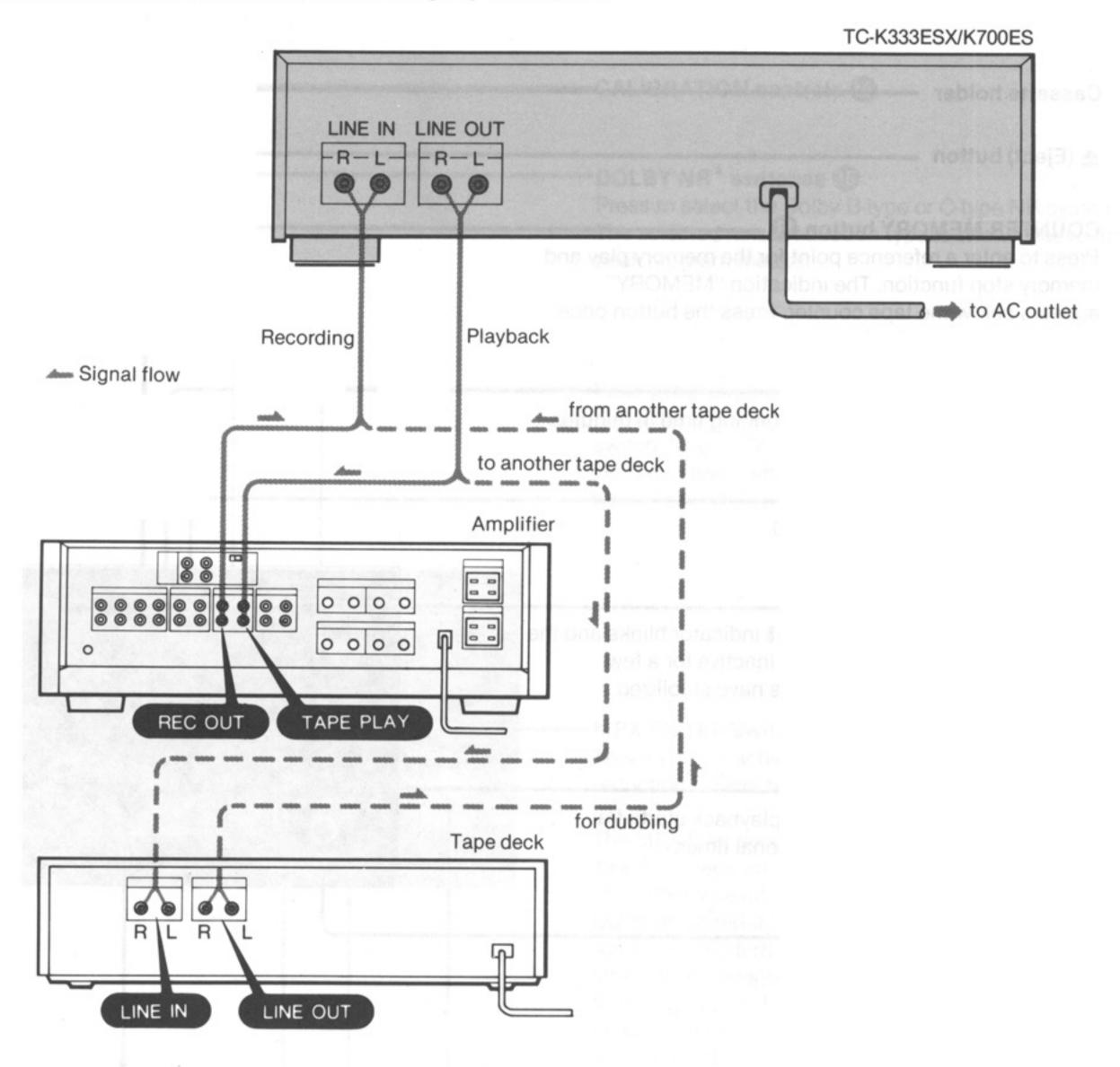
Use the supplied cables and make connections as shown in the illustration.
