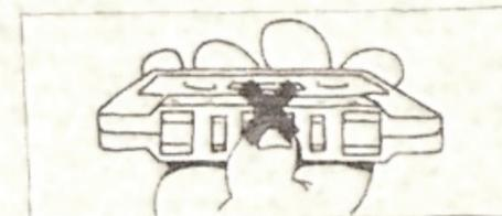
● Do not stick thick labels or tape on the cassette, as this may affect proper cassette alignment and prevent the tape from making proper contact with the heads.
