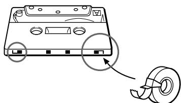
When you are using a type II or type IV tape, be careful not to cover the detector slots that the deck uses to determine the tape type.
