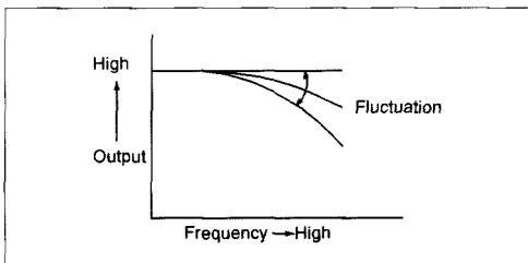
With the Dolby HX PRO system, the effective bias amount added to the bias current is controlled in millisecond units to greatly reduce distortion, improving linearity in high-range response and ensuring high-intensity recording with minimal distortion and noise.
