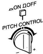
Push in the PITCH CONTROL button to activate Pitch Control function and turn the control clockwise to raise the pitch or counter-clockwise to lower it. You can adjust the pitch during playback on deck A or normal-speed dubbing (but not during RMS play or RMS dubbing).
