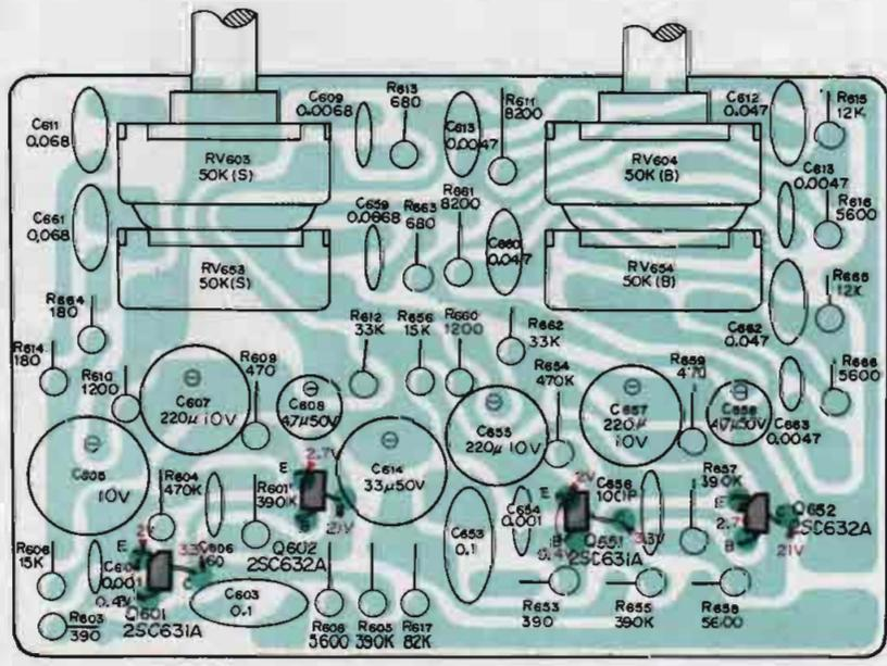
5-9. MOUNTING DIAGRAM – Power Supply Board –
