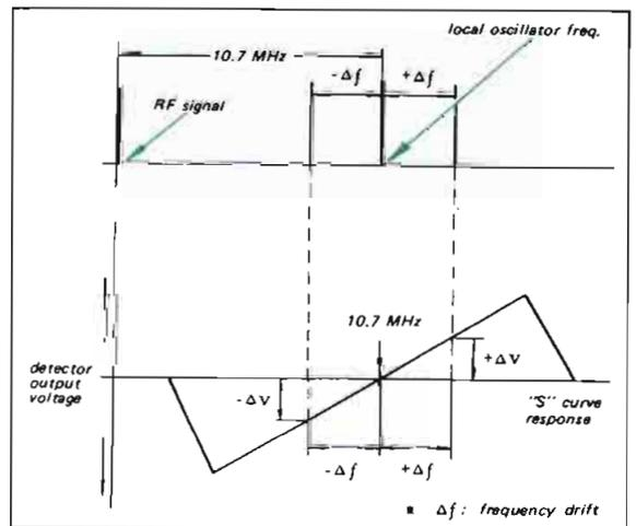
Fig. 1-1. Local oscillator's frequency drift and afc voltage relationship
