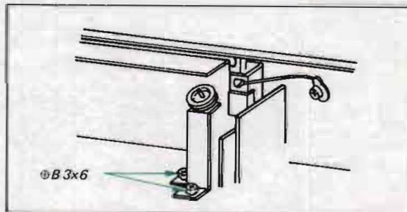
Fig. 2-16. Dial pulley bracket removal
