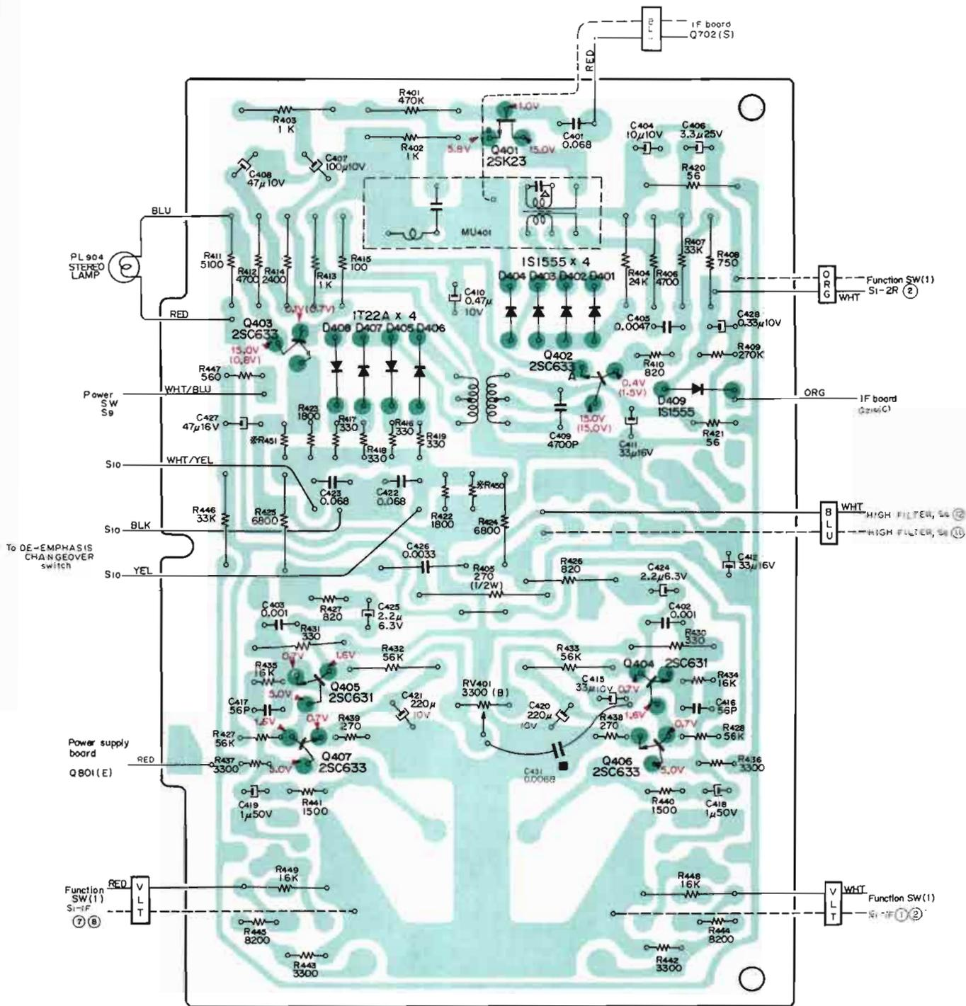
Note: ■ C431 is mounted on conductor side.
