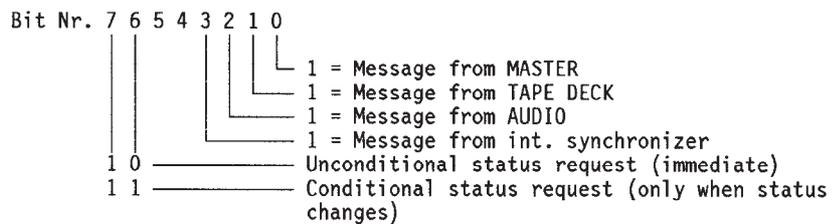
SBA, SBC (status request byte): SBA contains the base address, SBC the number of bytes of the requested status. CS (checksum): 2's complement notation of the sum of all data transmitted before the checksum, excluding STX.
