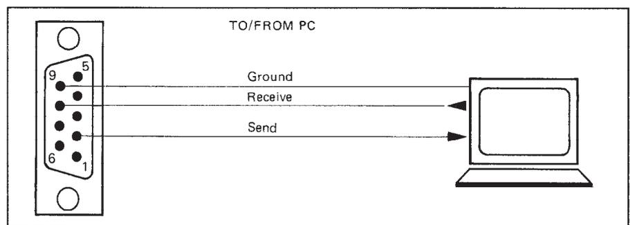
**Cab configuration for SAVE-, VERIFY-, LOAD-procedure with a PC**
