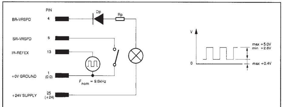
Circuit diagram for fader start with int. or ext. current supply
