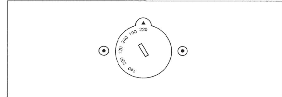
**Important:** Before you put the machine into service for the first time, make sure the setting of the line voltage selector on the back of the machine corresponds to the local line voltage. The following line voltages can be selected: 100, 120, 140, 200, 220 or 240 VAC,  $\pm 10\%$ , 50–60 Hz, For changing the setting, the machine must be completely disconnected from the power source. After the line voltage selector setting has been changed, also the power fuse (size 5x20 mm) must be changed.
