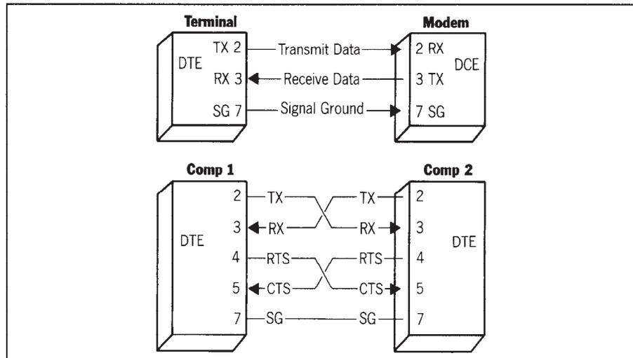
Fig. 9.1 Terminal-Terminal Connection
