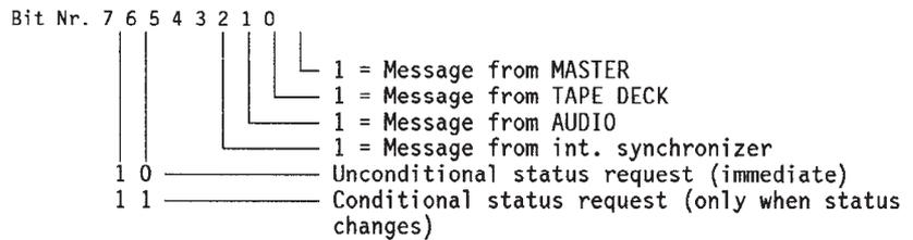
SBA, SBC (status request byte): SBA contains the base address, SBC the number of bytes of the request status.
