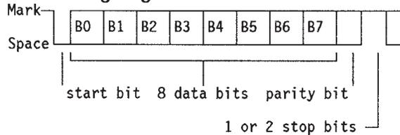
Odd or even parity and the number of stop bits (1 or 2) can be programmed.
