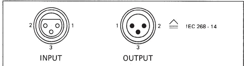
The balanced inputs and outputs are terminated on XLR sockets or connectors (pin assignment according to IEC recommendation 268-14).
