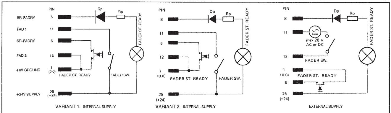
**Important:** If incandescent bulbs are used for status signalling, their inrush current must not exceed 0.3 A !
