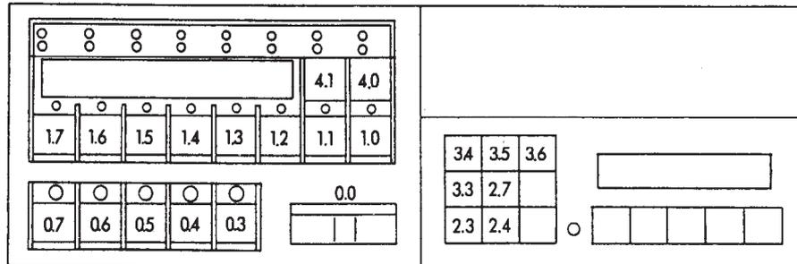
Key numbering of the serial remote control (Rem.)
