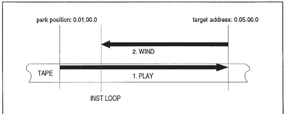
**INSTANT LOOP key determines the end of the loop**
